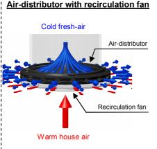
In extremely cold climate zones it can be advisable to use a recirculation fan. The latter can be ordered directly with the AD or be retrofitted any time.
