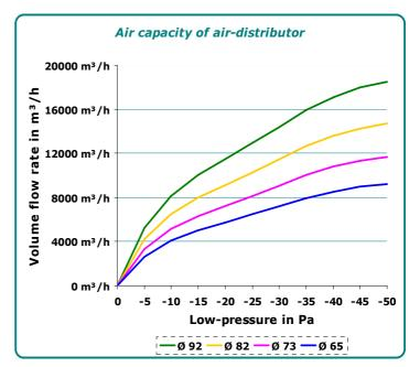
Fig.3a: Table: air capacity of the AD at maximum opening level
