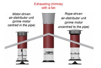
The air-distributor (AD) provides a steady fresh-air distribution in the livestock building. It is assembled just below the building roof and leads the fresh air from the outside through the roof area to the inside of the building. Here, the fresh air is subsequently delivered through the distributing disc and –ring.
